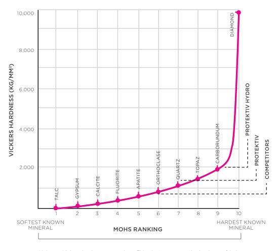
Mohs vs. Vickers hardness comparison: This chart compares the hardness of index minerals of the Mohs hardness scale (an integer scale) with their Vickers hardness (a continuous scale). Mohs hardness is a resistance to being scratched, while Vickers hardness is a resistance to indentation under pressure. The graph shows the great difference between the Vickers hardness of Carborundum and diamond - which are only one unit apart on the Mohs hardness scale.
